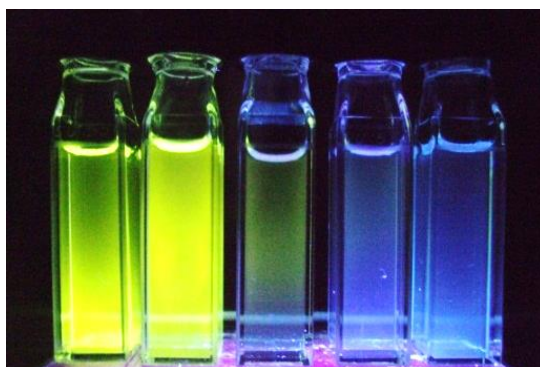
Fig. 9. Photographs of fluorescence of 2a upon irradiation with 365 nm light as an excitation light. The solvent is n -hexane, toluene, THF, methanol, and DMSO from the left.
